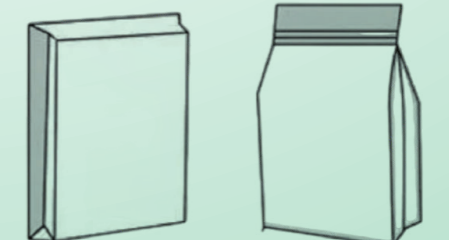
平底袋 (八边封袋) FAT BOTTOM BAG 拉链平底袋 (八边封袋) FLAT BOTTOM BAG WITH ZIPPER
